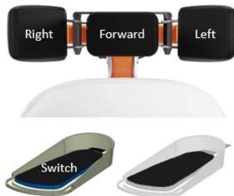
Figure 14. Drive with back head - Switch with one foot.
