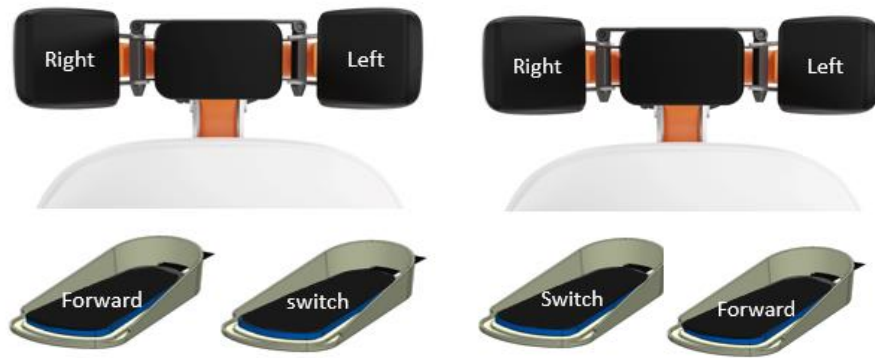
Figure 13. Drive with foot - Switch with foot configuration.
