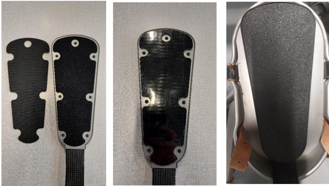
Figure 12. Velcro to attach foot pads to the wheelchair footrest.
