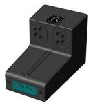
The remote button interface is an interface to connect up to 6 switches to the R-Net bus. The functions are programmable per switch via the R-Net PC program. Maximum 2 Remote Button Interfaces can be connected to the R-Net bus system. This allows you to connect up to 12 switches.
