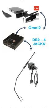
Rnet Input/Output module set up for interfacing CoMoveIT Smart with swing away arm.
