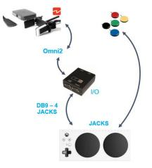
Rnet Input/Output module set up for interfacing CoMoveIT Smart with Xbox Adaptive.
